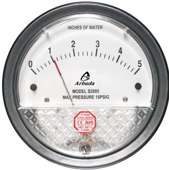
The Series E2000 is a low cost, diaphragm operated, differential pressure gauge. The S2000 can be used in applications for measuring positive, negative, or differential pressure with an accuracy of 2%. Standard applications include monitoring filter status, duct static pressure, room pressure, fan or blower pressure, paint booths, dust collectors, and cabinet purging along with many others.
