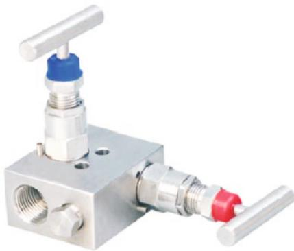
With threaded vertical port inlet and female outlet. The vent/test connection is positioned on the front side. The venting bonnet is positioned on the right hand side and the isolating bonnet on left hand side.
