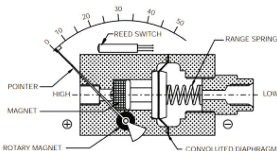
High and Low pressures are separated by a sensor assembly consisting of a magnet, piston, Teflon seal and a range spring. The difference in pressure causes the sensor assembly to move in proportion to the change against a range spring.
